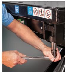
To tilt, thread jack screws located at the rear of lift table upward using allen wrench or allen socket until correct angle is met.
