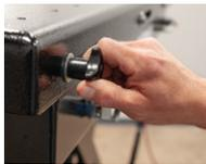
Platform easily locks and unlocks for fine adjustment of under vehicle placement.
